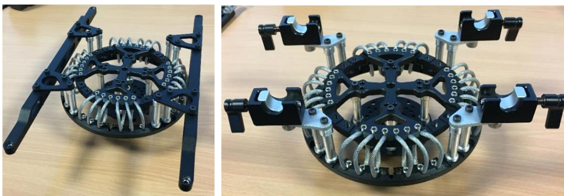
Figure 2: UAV mount options. Left picture: mount to be attached directly to M600. Right picture: quick release system to be attached to the rails of M600
