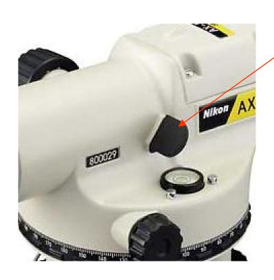
Allows easy viewing of the level bubble when on a tall tripod, which means more flexibility in set up location
